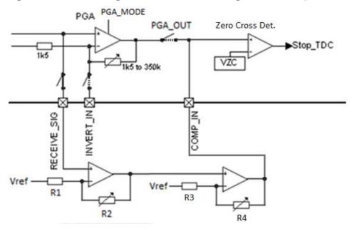
Figure 2: Schematic diagram of AS6040 with 2-stage external amplifier
