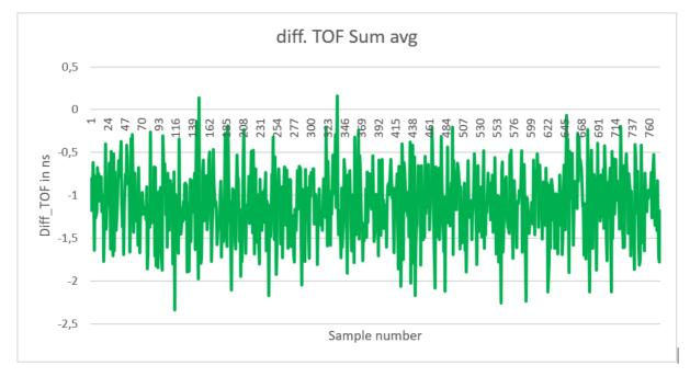
Figure 5: Measurement result with single amplifier of diff TOF. The standard deviation over 100 samples is around 410 ps.
