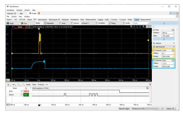
Figure 13: Pulse at GPIO3 after TOF Measurement Sequence
