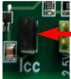
Figure 2.6: Measure power consumption
