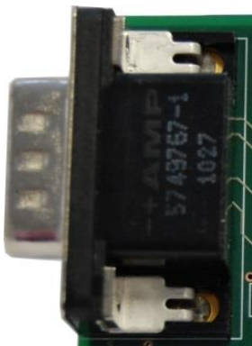
Figure 2.3: 15-pin VGA connector for power supply
