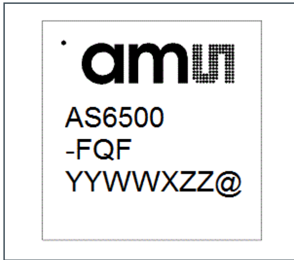
Figure 58: QFP48 Package Marking/Code
